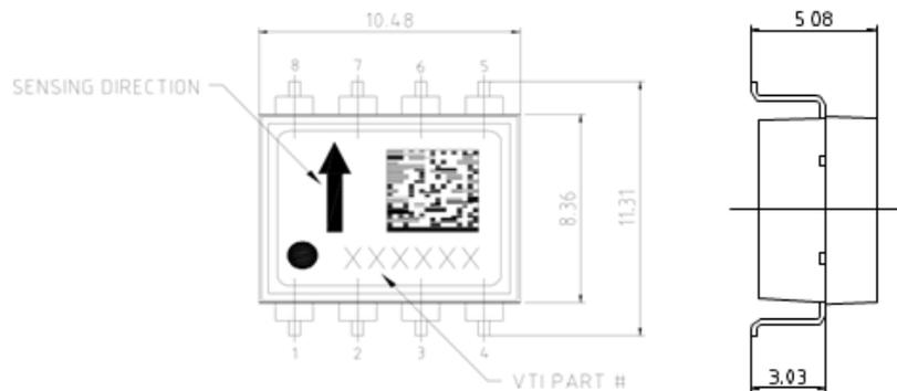
**Figure 8.** Mechanical dimensions (mm).
